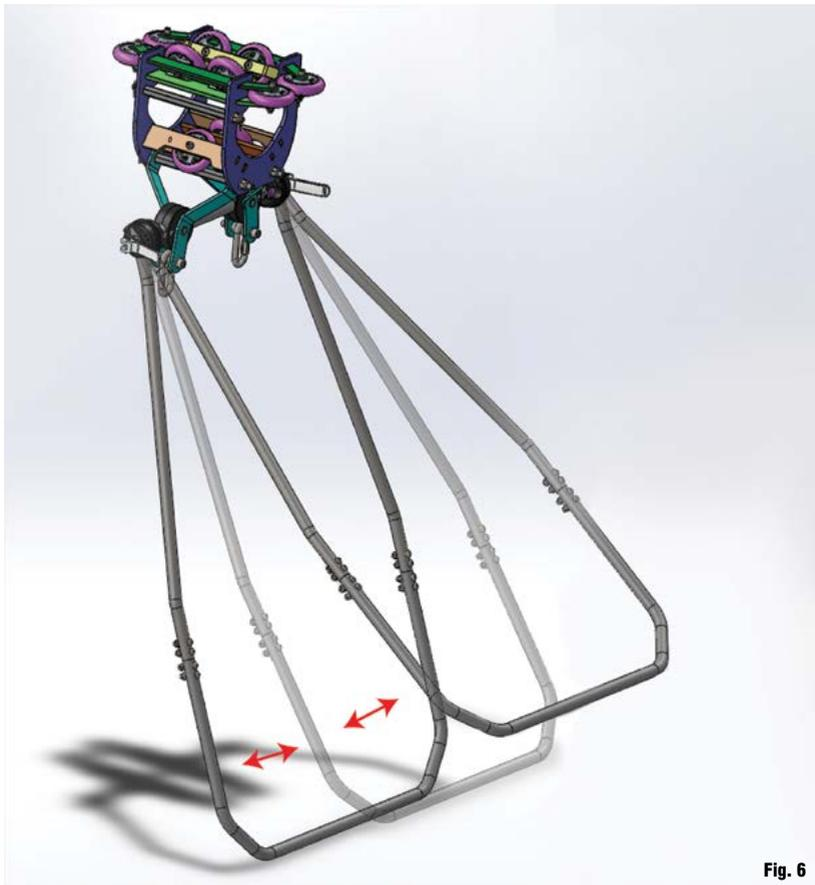
**4.** When the angle is set, it is important to firmly tighten and lock the handles because the ride causes mechanical vibrations that can potentially loosen the handles. The handlebar is safely constructed to block the handles from falling off even if they come loose during the ride but keeping them tight would prevent unwanted change in the angle during the Rollglider ride and would ensure the fun and exciting experience of your client.
