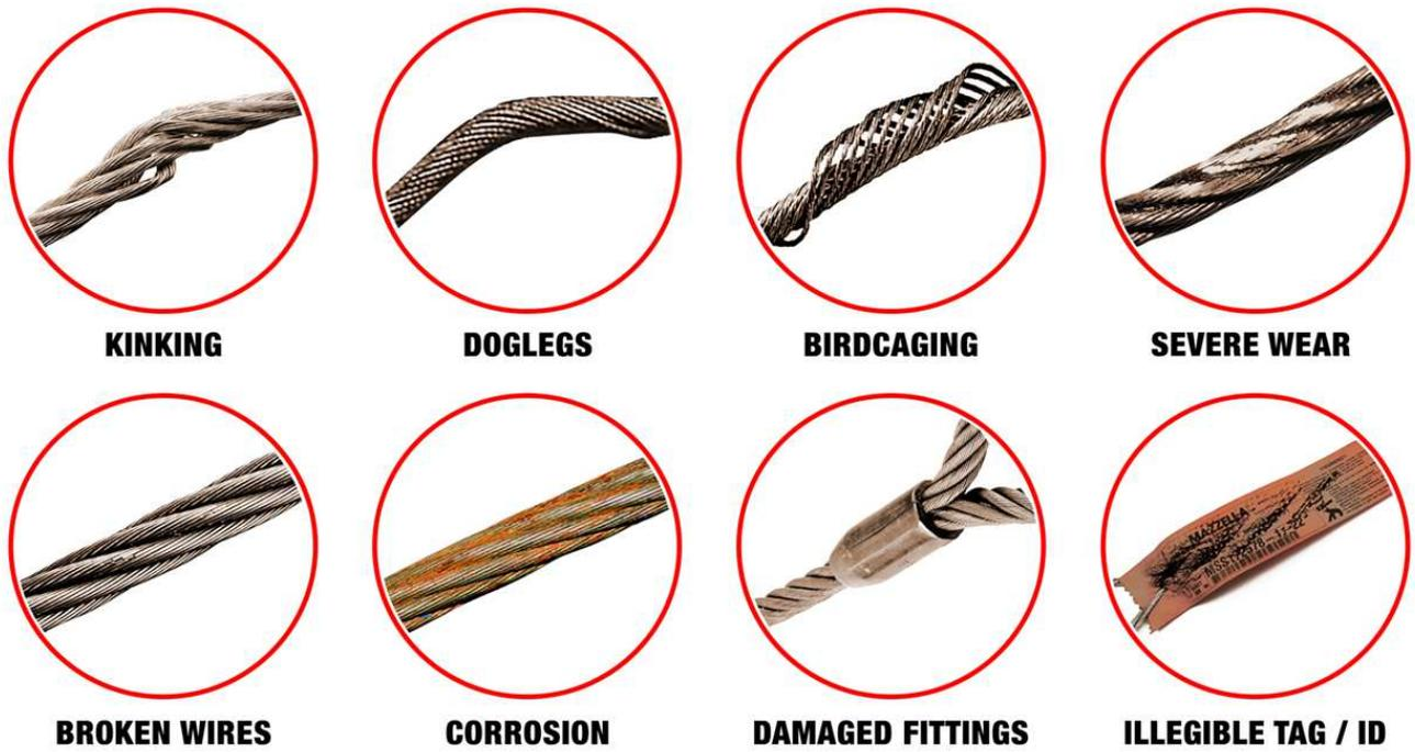
*Figure 6. Typical steel cable damages*
